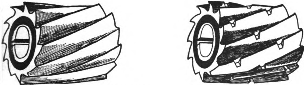
① Plain milling cutter with helical teeth. ② Helical cutter with nicked teeth.
